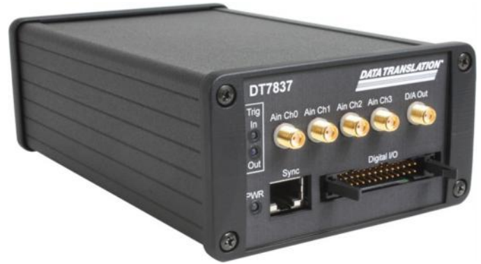
Figure 1. The DT7837 provides 4 IEPE input channels along with an embedded BeagleBone Black industrialized ARM processor for real-time processing and analysis of sound and vibration measurements. Compact, rugged metal enclosure measures 165mm x100mm x55mm.
